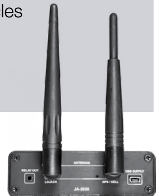
J-ALERT Rear Panel including Antennas, Relay Out, and USB Supply
